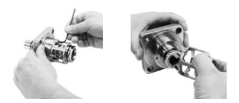
Figure 13: Removal of the PEV Plug Housing
