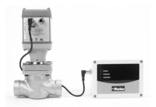
The PEV Backup Module is designed to bring the PEV electronic control valve to a user-defined position upon loss of power. The PBM can replace an upstream solenoid valve or user supplied uninterruptible power supply and offers a higher level of safety to the entire system. The PEV-PBM combination can be programmed to return to a full open, full closed, or defined position. Instructions on how to program the loss of power postion see the software parameters table on page 8 (level 1; section 07).
